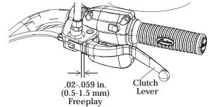
Verify that the safety switch activates properly. The engine should not start in gear with the clutch lever released.
