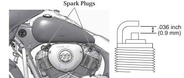
To prevent debris from entering the spark plug holes, use compressed air to clean the area around the plugs before removing them.
