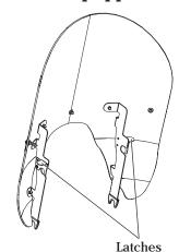
**WARNING!** Improper windshield installation can result in loss of control, accident and driving hazards for other motorists (if windshield falls from the motorcycle). Always make sure the windshield is fully seated before engaging latches.
