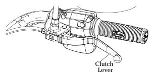
2. Freeplay (gap) is the amount of lever movement from the rest position to the point of cable resistance. Clutch lever freeplay should be 0.5-1.5 mm. Measure the gap between the clutch lever and the lever housing. See page 95. Adjust clutch lever freeplay if necessary.
