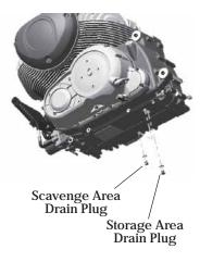
6. Reinstall the drain plugs. Torque to 15 ft. lbs. (20 Nm).
