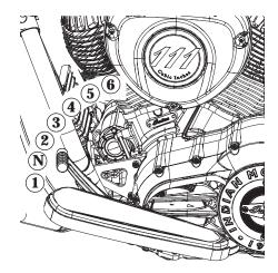
Press downward on the toe lever to shift to a lower gear. Lift upward on the toe lever to shift to a higher gear. Release the clutch lever after each gear shift. Shifting to neutral is easiest if the motorcycle is rolling slowly. To shift from first gear to neutral, gently lift the toe lever a half stroke.
