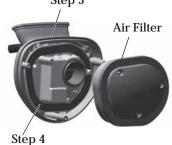
7. Reinstall the three screws. Torque to specification.
